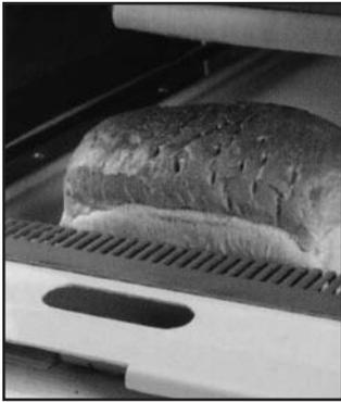
Available as an option, an automatic and retractable loaf pusher helps slice the last loaves.
